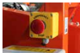
EMERGENCY PUSH BUTTON
