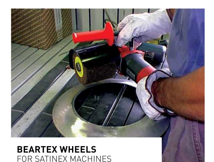
Beartex Satinex wheels provide a cushioned abrasive action which not only works well on flat areas, but is also ideal for use in finishing operations on uneven surfaces. These versatile wheels are used on portable machines.
