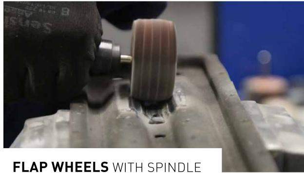
Flap wheels conform to intricate shapes and contours. Designed to deliver a consistent finish with a uniform rate of cut, they wear away evenly and without
