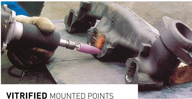
The Norton vitrified mounted points range provides quality and efficiency in grinding operations. The high quality grain ensures a perfect surface finish with metallographic integrity. For small jobs or high volume foundry and casting operations, or for tool room or aerospace industry applications, Norton vitrified mounted points cut cooler, and provide up to 30% higher metal removal rates.
