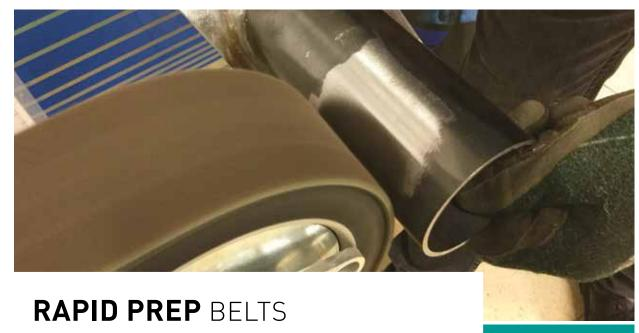
Norton non-woven belts are a combination of strong synthetic mesh and quality abrasive, bonded together by a smear-resistant adhesive. The open construction of non-woven material enables aggressive cutting action and improved surface finish while maintaining its non-loading feature. Ideal product to provide a great finish or remove burrs without gouging or undercutting the workpiece.
