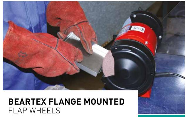
Formed by mounting sheets of Beartex around a centre core. The tightly packed piece forms the spokes of a wheel. This construction makes flap wheels the most conformable of all Beartex wheels providing a cushioning action which is ideal for use on uneven or irregular surfaces, as well as flat areas.
