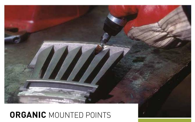
Produced specifically for demanding applications, Norton organic mounted points work harder for you. With stock removal that's twice as fast and product life that's up to four times longer than their conventional aluminium oxide counterparts, organic mounted points increase productivity and clean more parts in less time, reducing your overall process cost.
