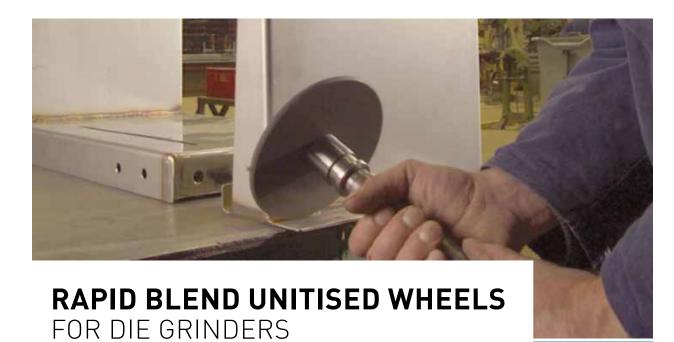
Unitised wheels are made from compressed and bonded layers of non-woven abrasive for maintenance operations where an efficient, cost-effective solution is needed for deburring, polishing, cleaning and finishing composites. The uniform construction maintains part tolerance and prevents cutting and gauging. Rapid Blend can be used on a variety of shapes and contours, wheels hold their shape well and don't need to be dressed as often. Wheels are also non-metallic so won't contaminate the workpiece.
