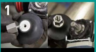
Remove the metallic spindle and screw the adaptor to use the rubber back-up directly on the angle grinder.
