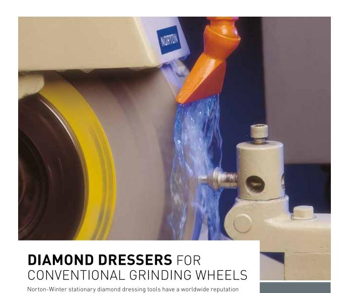
for quality and technology. Ideal for profiling and straight dressing of all conventional grinding wheels.
