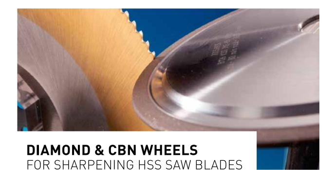
HSS saw blades are one-piece saws that are ground from one solid piece of metal. For this process HSS saws require special grinding machines.
